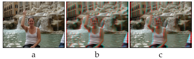
Fig. 6: Comparison showing the effect of incorporating our 3D model \mathcal{M} into the stereoscopic conversion. a) Original image, b) result computed using a planar approximation to the background, c) result computed using \mathcal{M} . In the latter case, the rocks on the right can be seen at their correct depth level. Please view zoomed-in on screen for best results.
