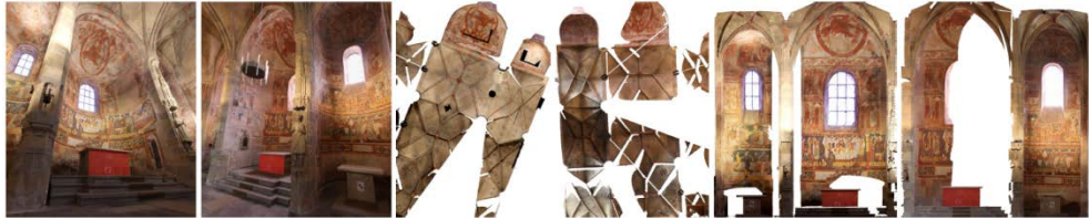
Fig. 2: (Left:) Images taken from 2 different scanner positions, which naturally exhibit a wide baseline. Feature matching and thus registration from these images fails in most cases. (Middle, right:) Generated salient direction rectified renderings which are subsequently used for our automatic registration.
