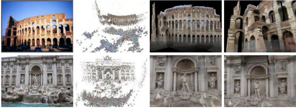
Fig. 5: (Left:) Sample input images obtained from Flickr; (2nd left:) Local sparse SfM reconstruction. (Right:) Dense, textured 3D model seen from 2 different views (FRAHM et al. 2010).
