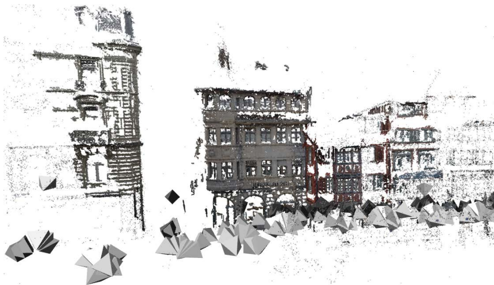
Fig. 1: Part of an urban reconstruction computed via Structure-from-Motion and dense reconstruction obtained solely from images. The gray pyramids visualize camera location and orientation for captured photographs.
