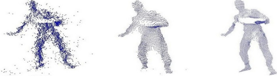
Figure 5. Comparison of point cloud smoothing using bilateral filtering and our modified LOP algorithm. From left to right: input; after Bilateral Filtering; after our modified LOP.
