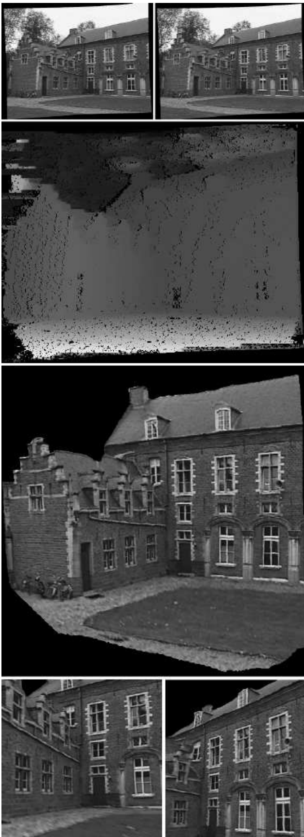
Figure 10: Images from the 'Arenbergkasteel' Original left and right image are shown at the top. The disparity map is presented in the middle together with a 3D model and 2 details of this model.
