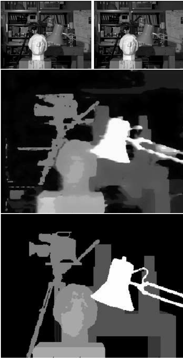
Figure 12: Tsukuba dataset for testing accuracy. Original left and right image are shown at the top. The disparity map is presented in the middle. The ground truth can be found at the bottom.
