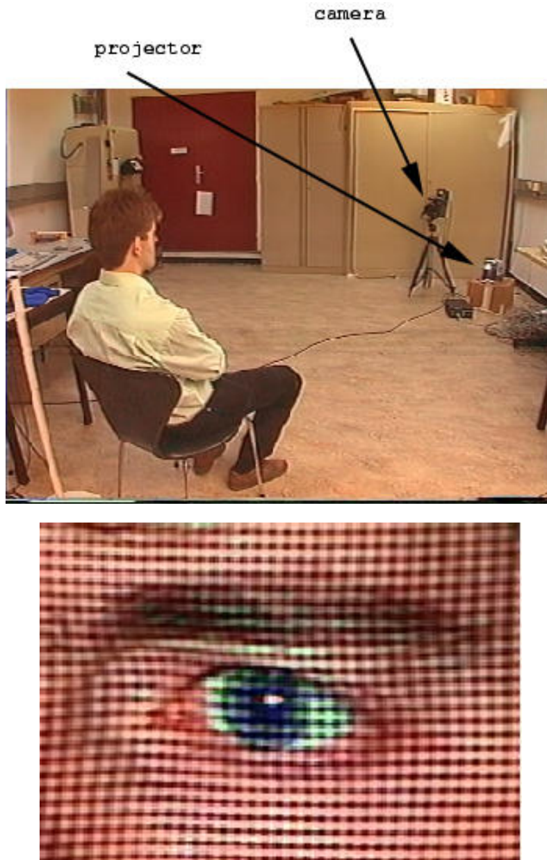
Figure 7: Top: The active system only consists of a normal slide projector and camera, and a computer. The camera takes an image from a direction that is slightly different from the direction of projection. Bottom: A regular square pattern is projected on the scene, as seen in this detailed view. In this case, the grid covers the complete face. 3D coordinates are calculated for all the line intersections, resulting in the simultaneous measurement for thousands of points.
