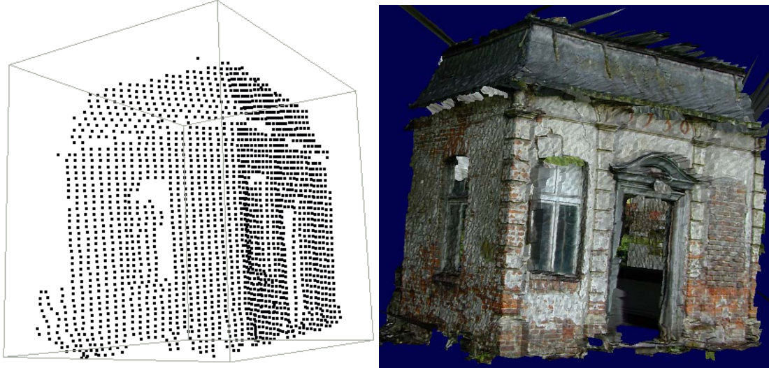
Fig. 6: 3D point reconstruction (left) and textured 3D reconstruction (right)
