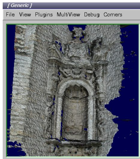
Fig. 9: 3D reconstruction obtained using a fully automatic reconstruction approach
