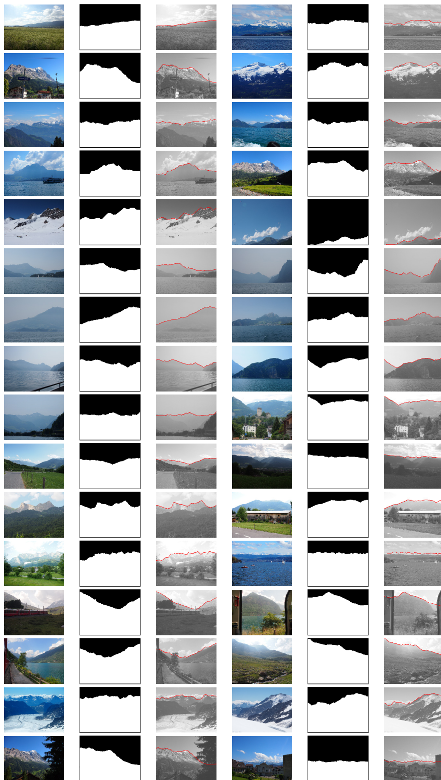
Fig. 8 Sample Results: First and fourth column are input images. Second and fifth column show the segmentations and third and sixth column show the query images augmented with the skyline, retrieved from the database. The images in the last five rows were segmented with help of user interaction.
