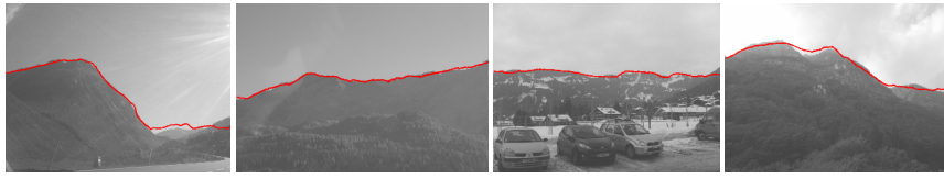
Fig. 9 Some incorrectly localized images. This usually happens to images with a relatively smooth skyline and only few distinctive features. The pipeline finds a contour that fits somewhat well, even if the location is completely off.
