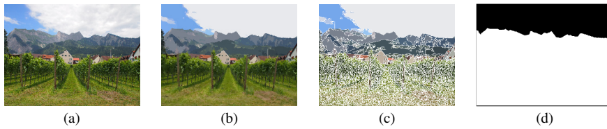
Fig. 2 Superpixel based segmentation: (a) Input image. (b) MeanShift filtered image. (c) MeanShift region boundaries. (d) Final segmentation.
