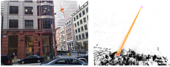
Figure 3: A sample query image with a pose that has more than 30 inliers even though it is obviously wrong. Inliers are only found in a small region of the image, forcing pose estimation to place the camera far away from the scene. Note that structure-based localization approaches typically use a threshold of 12 inliers to detect bad poses.
