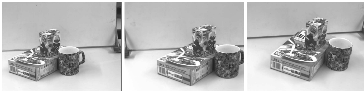
Figure 5: The 3 images that were used to build a Euclidean reconstruction. The camera was translated between the first two views (the zoom was used to keep the size more or less constant). For the third image the camera was also rotated.
