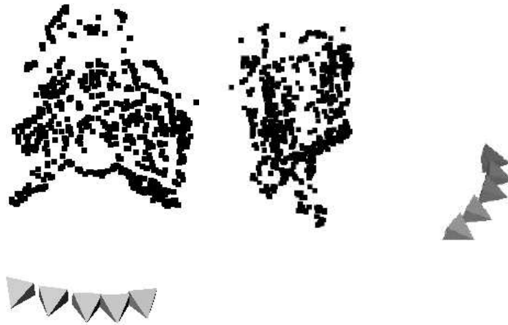
Figure 11. Reconstruction of interest points and cameras. The system could automatically reconstruct a realistic 3D model of this complex scene without any additional information.
