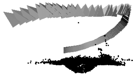
Figure 10: The reconstructed interest points and camera poses recovered from the BRT sequence.
