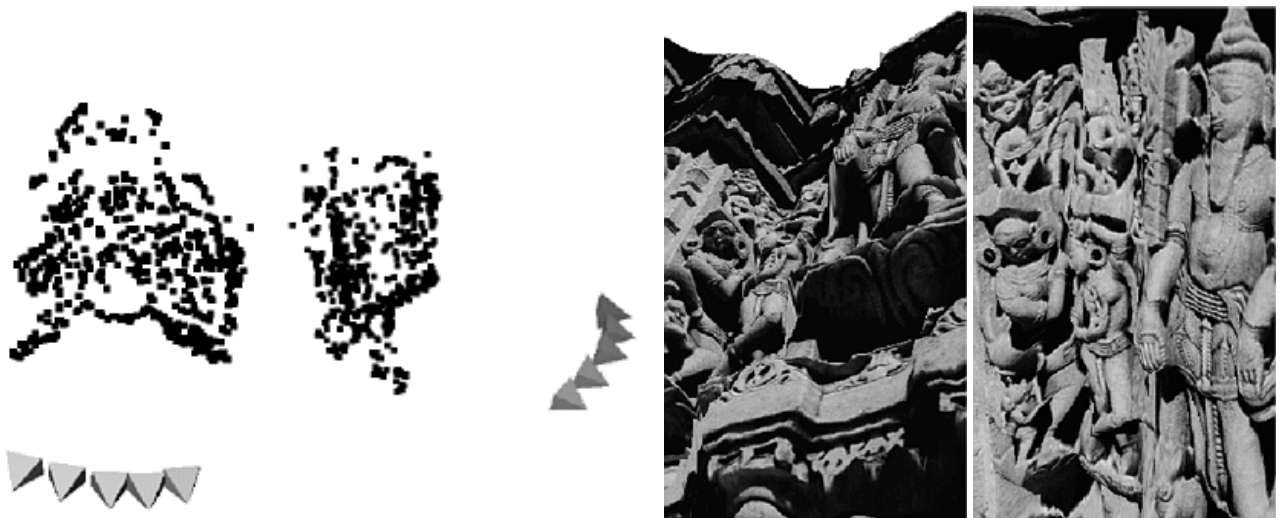
Figure 9: Reconstruction of interest points and cameras (left), two detail views of the reconstructed model (right).
