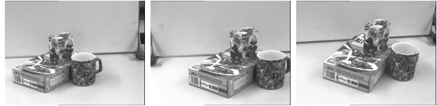
Figure 1. The 3 images that were used to build a Euclidean reconstruction. The camera was translated between the first two views (the zoom was used to keep the size more or less constant). For the third image the camera was also rotated.
