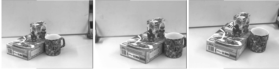
Fig. 3. The 3 images that were used to build a Euclidean reconstruction. The camera was translated between the first two views (the zoom was used to keep the size more or less constant). For the third image the camera was also rotated.
