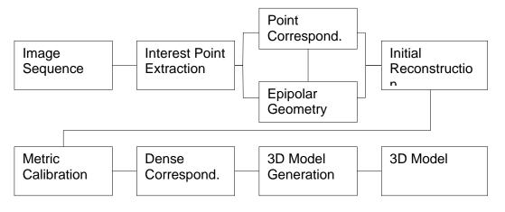
Figure 4 Overview of 3D-model acquisition from multiple views
