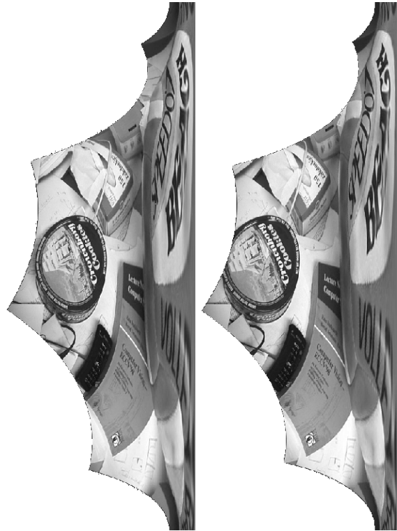
Figure 9. Rectified pair of images of the desk. It can be verified visually that corresponding points are located on corresponding image rows. The right side of the images corresponds to the epipole.
