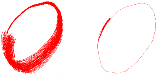
Fig. 7. (Left) Particles trajectory just before loop closure. (Right) Particles trajectory after loop closure. The particles converged upon loop closure.
