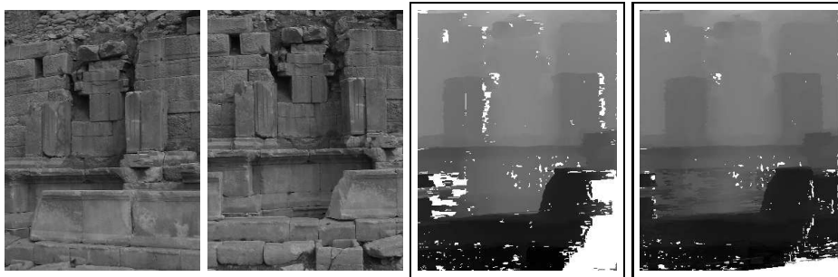
Fig. 7. Left: First and last image of sequence. Right: Depth maps from the 2-view and the 5-view estimator (from left to right) showing the very dense depth maps.
