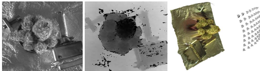
Fig. 3. Spherical motion. Left: One of the input images. Center: Dense depth map of scene. Right: 3D surface model and calibrated camera grid of spherical scene.
