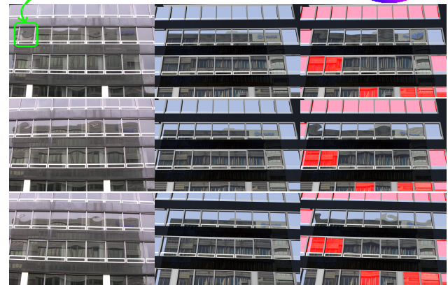
Figure 11. Estimated height field and normal map for a real facade sequence (see Sec. 4 and attached video for explanations). 1st column shows still frames from the original sequence, 2nd with perfect mirrors, 3rd our reconstruction (red windows do not have a computed normal map)
