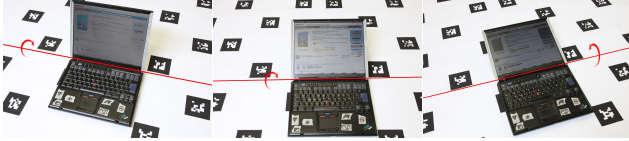
Figure 2: Our method accurately recovers the rotation axis \mathbf{a} (in red) of a laptop opening and closing its screen from pure imagery data taken by a moving camera. This articulated motion has signature (2, 0) and is thus equivalent to the motion of a door, for example.
