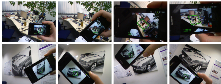
Fig. 6. Tracking on a mobile phone. The upper row shows tracking a non planar surface while the lower row shows tracking a planar scene.
