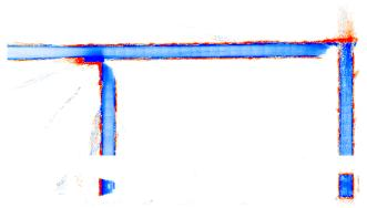
Fig. 3. Horizontal and vertical slice through the occupancy grid. The blue colors denote negative and the red colors positive values. The absolute value of the weights is visualized by the saturation of the colors. (best viewed in color)
