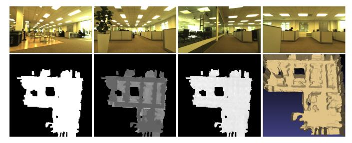
Fig. 15. Top row: 4 out of 518 input images. Bottom row: labeling result, regularized floor and ceiling height level with  $L_1$ -norm total variation, 3D model of the whole office data set.
