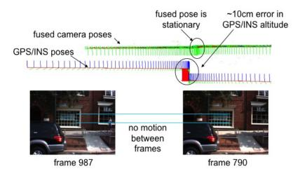
Figure 3: Correction of GPS and INS track through fusion with local correspondences. The top shows a view on compensated 3D camera path (green) and measured GPS and INS path (blue). Each camera is shown through its 3D coordinate frame located at the optical center of the camera. Note the camera is not moving between frame 790 (bottom left) and frame 987 (bottom right) as shown through the two vertical lines. The erroneous GPS track reports a 10 cm vertical motion.
