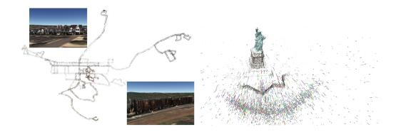
Figure 1: Left: an overview model of Chapel Hill reconstructed from 1.3 million video frames on a single PC in 11.5 hours. Right: a model of the Statue of Liberty consisting of 9025 cameras registered out of 47238 images downloaded from the Internet.
