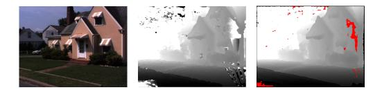
Figure 5: Our depth map fusion method combines multiple stereo depth maps (middle image shows an example depth map) to produce a single fused depth map (shown on the right) with greater accuracy and less redundancy.
