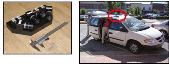
Figure 1. Example of a multi-camera system on a vehicle
