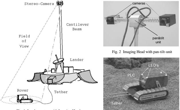
Fig. 1 Lander system with Imaging Head and Nanokhod Rover
