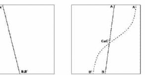
Fig. 8 DEM generation in detail: left and right disparity image with the projection of the vertical line and the "shadow"
