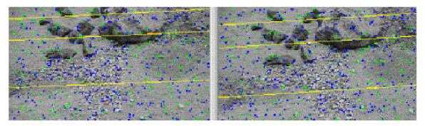
Fig. 5 Epipolar geometry of an image pair
