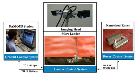
Fig. 4 Communication links between the subsystems
