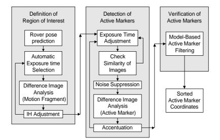
Fig. 16 Control flow of AM detection
