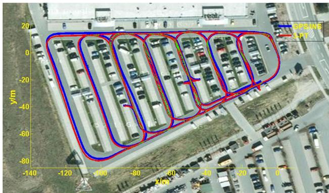
Fig. 9. Pose-graph for ParkingGarage02 dataset after pose-graph optimization (red) compared with trajectory from GPS/INS (blue) overlaid on the satellite image.
