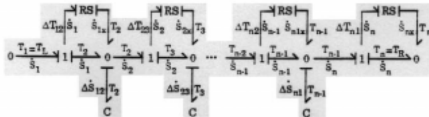
Figure 8.11. Corrected causal bond graph for the diffusion chain
