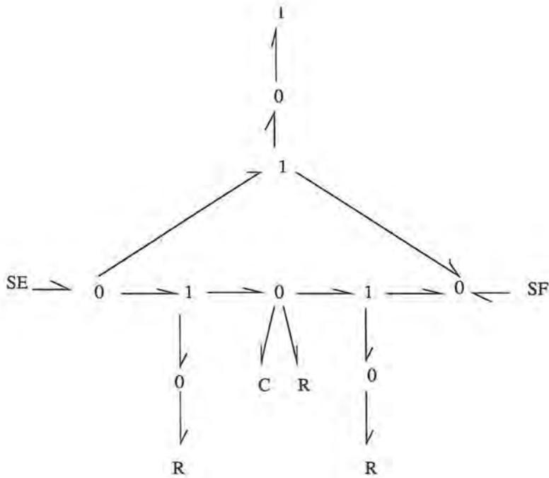
Figure 1.3: bond graph for a passive circuit ready for implementation in Dymola
