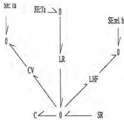
Figure 7.2: bond graph for the energy balance of a plant under steady state conditions
