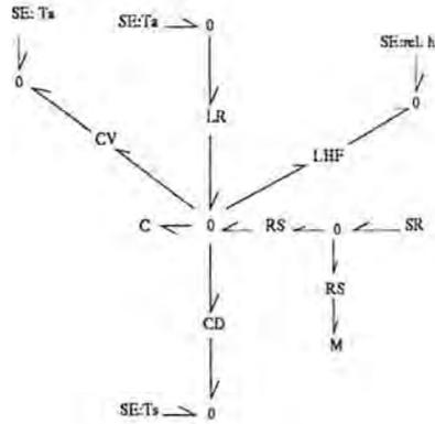
Figure 7.1: bond graph for the energy balance of a plant
