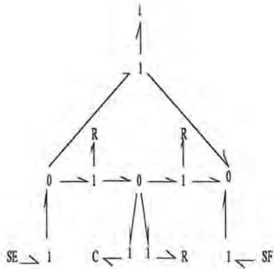
Figure 1.2: bond graph for a passive circuit
