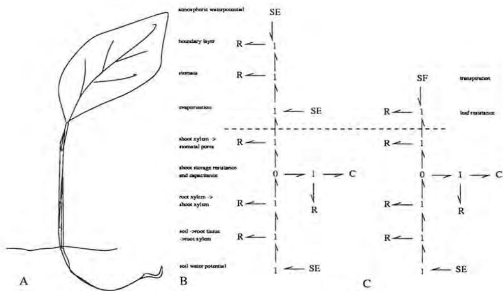
Figure 5.1: bond graph of a simplified plant
