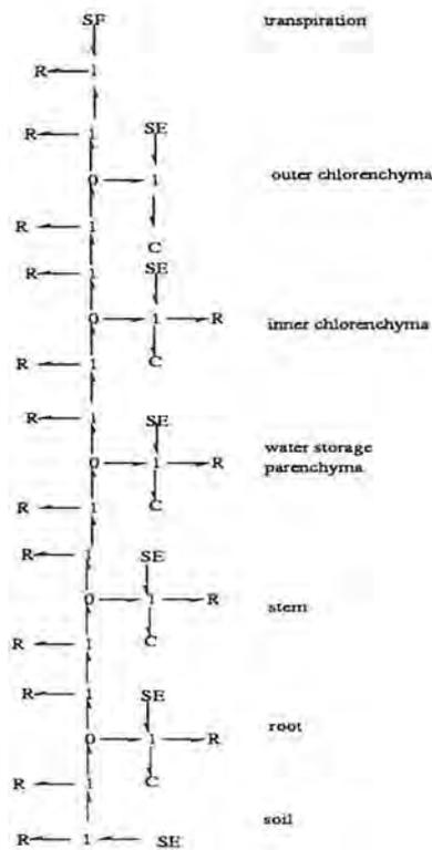
Figure 6.2: bond graph of tissues hydraulic architecture
