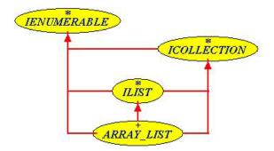
Fig. 4. Inheritance hierarchy of the .NET arrayed list class
