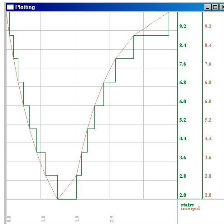
Figure 3.7: The result of the model in Figure 3.1. Once plotted as a stair function, once with the output points linearly connected.
