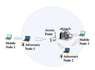
Fig. 2. Relay Attack on Network Access. Mobile Node 1 cannot directly connect to the Access Point because it is out of range. Similarly, Mobile Node 2 cannot directly connect to the AP due to an obstacle. However, the Attacker Nodes can act as relays between the Mobile Nodes and the Access Point, misleading them they can communicate directly, and thus control the communication.
