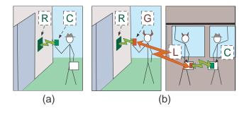
Fig. 1. RFID Access Control. (a) Normal operation: a legitimate user opens the door controlled by an RFID reader (R) using his RFID card (C). (b) The attack: the *leech* (L), next to the RFID card owner, and the *ghost* (G), next to the RFID reader, use a long-range link to relay transmissions between the card and the reader. As a result, the reader is misled to believe that the legitimate card is in its physical neighborhood and opens the door.
