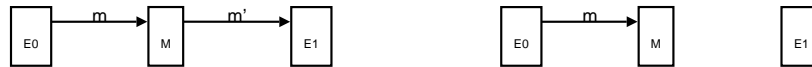
Fig. 3. A message m from endpoint E_0 to endpoint E_1 is forwarded (left) or dropped (right) by the midpoint M .
