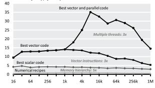
**Fig. 1**. Performance of four single precision implementations of the discrete Fourier transform. The operations count is roughly the same. *The labels in this plot are too small.*
