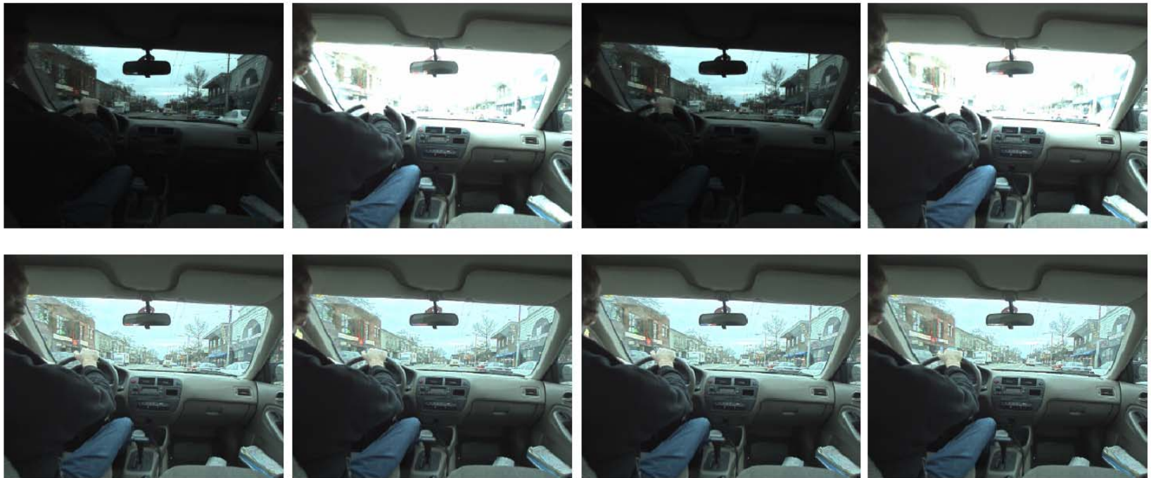
Figure 1: High dynamic range video of a driving scene. Top row: Input video with alternating short and long exposures. Bottom row: High dynamic range video (tonemapped).
