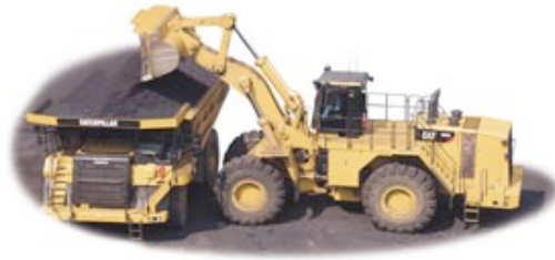
Figure 5.1. An FEL (Front-End Loader) Loading a Hauling Truck.
