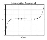
Figure: Interpolation polynomial used for extrapolation
