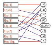
$U_0 = f(t)$  $i_{R} = \frac{1}{R_{L}} \cdot u_{2}$  $u_d = m_o \cdot s$  $u_1 = u_0 - u_d - u_2$  $\mathbf{i_0} = \frac{1}{R_i} \cdot \mathbf{u_1}$  $s = \frac{1}{1 - m_o} \cdot i_0$  $i_{C} = i_{0} - i_{R}$  $\frac{du_2}{dt} = \frac{1}{C} \cdot i_C$
