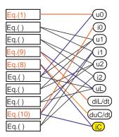
$$\begin{array}{lllll} 1: & u_0 & = & f(t) \\ ?: & u_1 & = & R_1 \cdot i_1 \\ ?: & u_2 & = & R_2 \cdot i_2 \\ 9: & u_L & = & L \cdot \frac{d_L}{dt} \\ 8: & i_C & = & C \cdot \frac{du_C}{dt} \\ ?: & u_0 & = & u_1 + u_L \\ ?: & u_C & = & u_1 + u_2 \\ ?: & u_L & = & u_2 \\ 10: & i_0 & = & i_1 + i_C \\ ?: & i_1 & = & i_2 + i_L \end{array}$$
