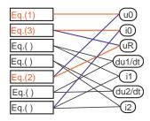
▶ The constraint equation has indeed disappeared. After partial causalization of the equations, we are now faced with an algebraic loop in four equations and four unknowns, a situation that we already know how to deal with.
