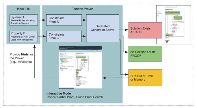
Figure 1. A high-level view of interaction with Tamarin.
