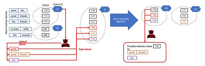
Figure 2: How an attacker extracts private information from FLoC. First, the attacker takes a cohort ID  $\gamma$  and then uses the GAN-IP attack to create fake browsing histories whose SimHash contains  $\gamma$  as prefix. These SimHashes make the cohort decomposable, so FLoC's clustering algorithm divides the cohort into smaller cohorts. The attacker exploits the fake histories to infer websites visited by real users.
